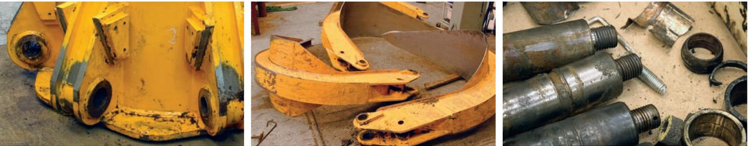
Part of the crown without the arms. Note the deformation of the materials and remains of the damaged mounting.
