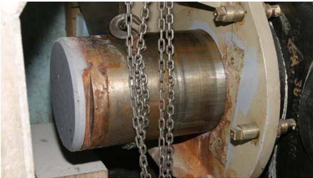
The existing shaft is removed in order to repair the hydraulic cylinder. Double sided gap in the mountings is discovered. Alternative corrective action is to replace both the cylinder mountings or replace the shaft with the Expander system.
